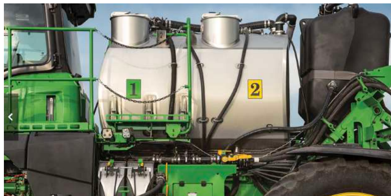
John Deere See & Spray Ultimate Dual-tank configuration Source: John Deere
